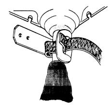
The Sicame Consumers Earth Bonds have been extensively tested both in our own laboratories and by independent authorities. Resistance values measured on bonds attached to a twin 0.0225 sq in (14.5mm²) PILC cable sheath before and after 2000 load cycles were as follows:-
