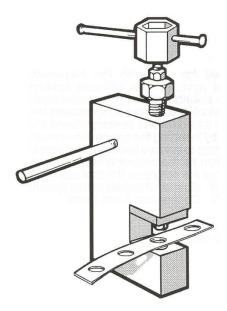
The Sicame Piercing Tool is hand-operated and designed to cut holes in metal strip on site. Each tool is supplied with a detachable holding handle and operating spanner and is suitable for use on steel, copper and aluminium.
